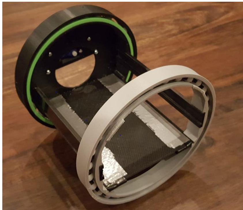
Figure 4-14 – Completed payload housing with front and back bearings, bottom panel, and axle rails
