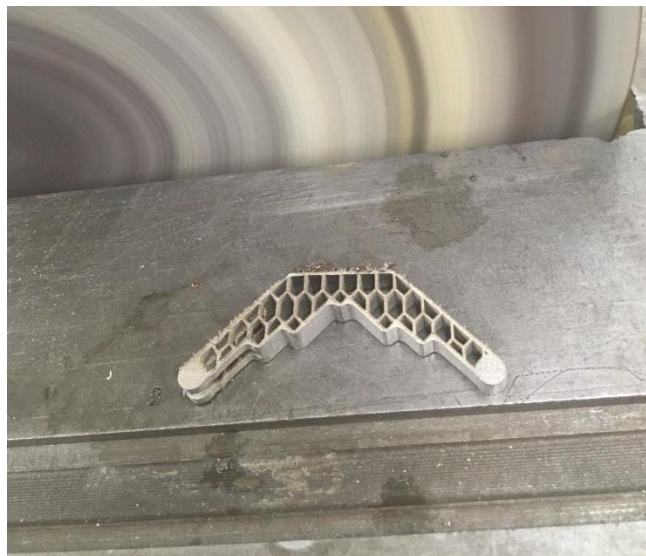
Post work grinding on the control arms
