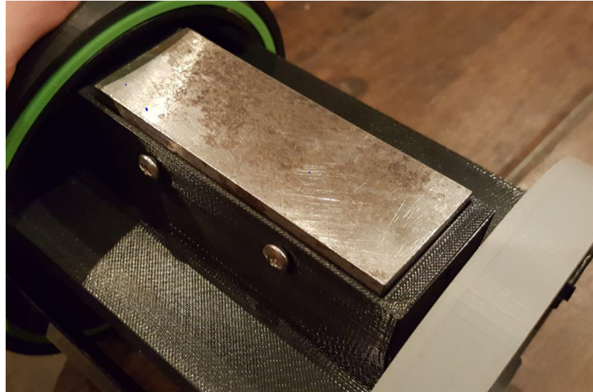
Figure 4-13 – Counterweight attached via #8-32 screws to the bottom platform of the payload housing
