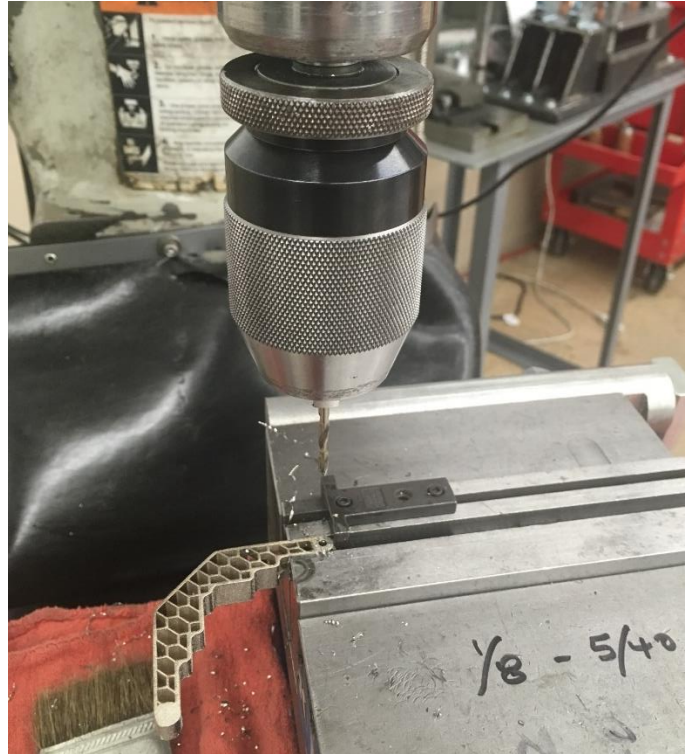
Post work, drilling out holes to be tapped
