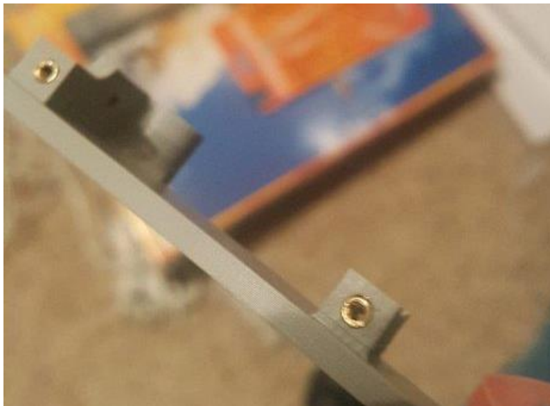
Figure 4-8 - #2-56 brass threaded inserts pressed into the plastic of a rover side panel
